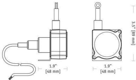
The SP2 String Pot is a compact, economical and water resistant device that utilizes a flexible cable, a spring-loaded spool, and a potentiometer to detect and measure linear position.
