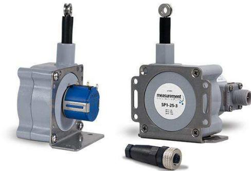
This compact stringpot with "voltage divider" output, provides ease-of-use and flexibility for measurement ranges up to 50 inches. Made of rugged polycarbonate, the SP1 fits in small spaces, doesn't need perfect alignment and ships with a stainless steel mounting bracket to let the user easily orient this sensor in just about any direction imaginable.
