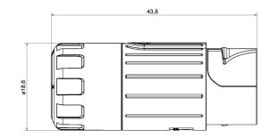
Main Dimensions Extension \*for max. wire cross-section pay attention to the cross-section of used contacts
