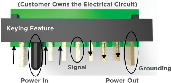
The diagram shows a cross-section of a connector with several pins. From left to right: a tall pin labeled 'Keying Feature', a group of three pins labeled 'Power In' with upward arrows, a single pin labeled 'Signal' with a downward arrow, a group of three pins labeled 'Power Out' with downward arrows, and a tall pin labeled 'Grounding' with a downward arrow.
