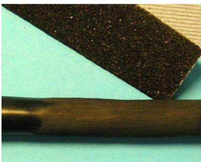
Figure 1 Degreased and abraded cable jacket
