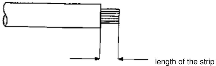
appropriate length: the length of wire barrel of used contact +0.5~1.0mm
