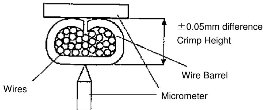
(4) Modified Micrometer for Measurement of Crimp Height
