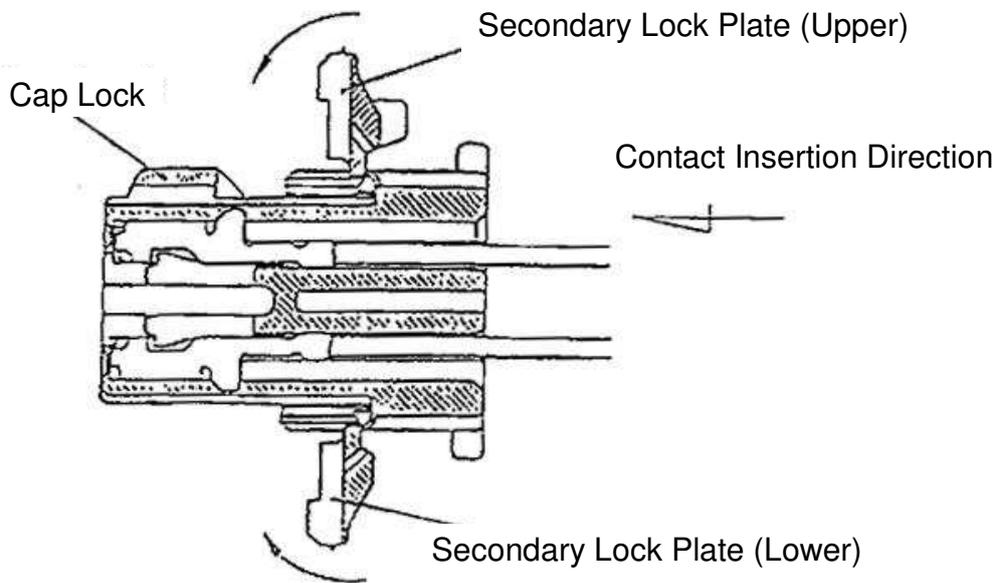
(1) After completing all contacts insertion, rotate each Secondary Lock Plate and then press both sides of Secondary Lock as shown two solid arrows in below figure at the same time until click sound is made.
