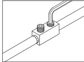
2. a. Insert conductors into connector.
