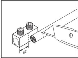
1. Remove insulation equivalent to half the connector length.
