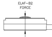
B0, B1 & B2: SPHERICAL CONTACT ON THE TOP AND FLAT SURFACE ON THE BOTTOM
