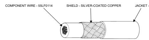
JACKET - ULTRA LOW FLUORIDE, RADIATION-CROSSLINKED, MODIFIED ETFE
