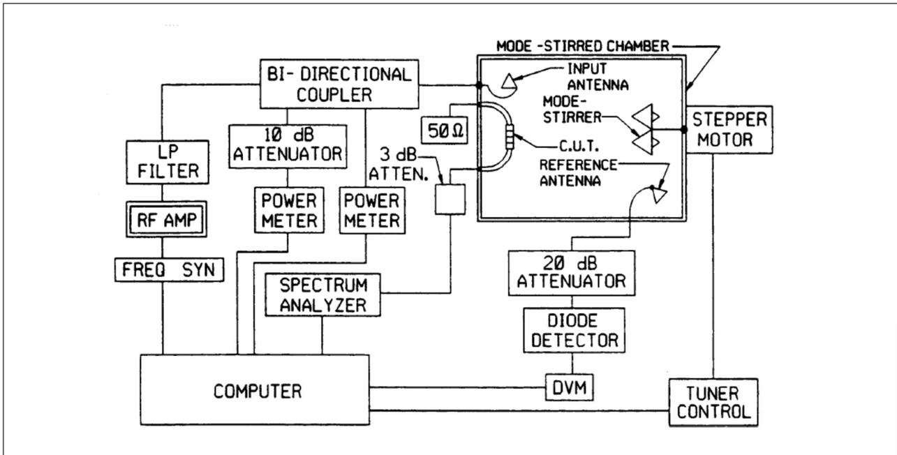
Figure 1 – Mode stirred shielding effectiveness measurement system
