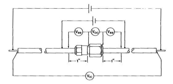
NOTE: (a) VBB is shield to body measurement. VOC is outer contact measurement. VIC is inner contact measurement.
