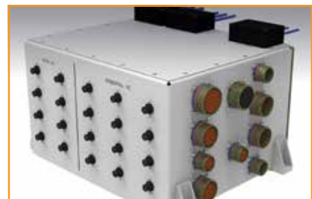
Primary and secondary 115 VAC, 400 Hz PDU using HARTMAN compact 200 A, 3-phase contactors and CII midrange relays
