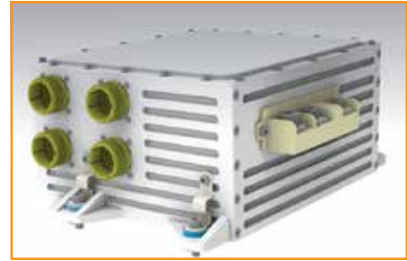
270 VDC EDU incorporating KILOVAC MAP series primary and secondary distribution contactors in a compact LRU enclosure
