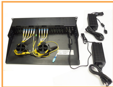
SuperChassis Back View - Fiber Management Tray
