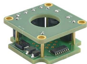
Subassembly Module with Selection of TVS Surface Mount Packages
