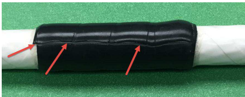
Unacceptable – evidence of adhesive on the top layer (arrow) – reverse installed.
