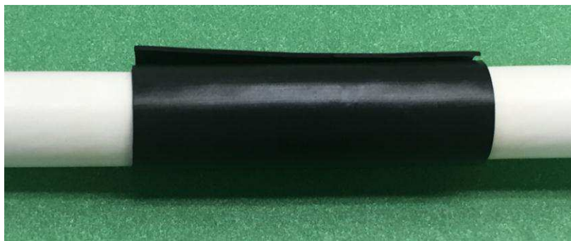
Unacceptable – incomplete bonding from insufficient heating (time or heat)
