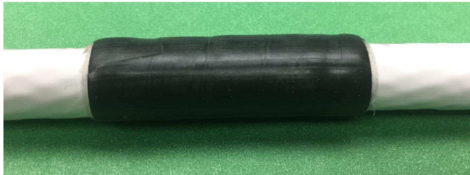
Acceptable – visible adhesive at both ends of the repair sleeve.
