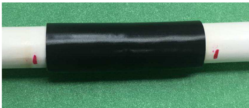
Unacceptable – no evidence of adhesive flow at the ends – insufficient heating
