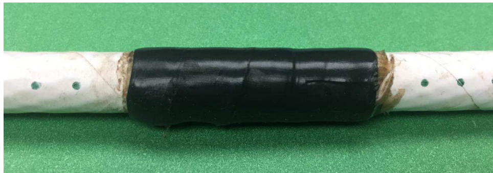
Unacceptable – darkened adhesive at and baked on PTFE tape adhesive residue – overheating.
