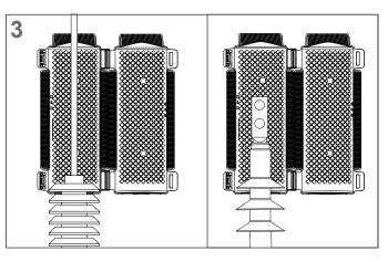
When using the cover on a recloser, position the cover between the first and second skirt.
