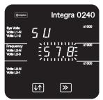
Initially all the digits of the current value will be flashing and the decimal point position illuminated. This is to indicate that initially the "multiplier" must be selected, pressing "\$\psi\$ Adjust" will move the decimal point position to the right.
