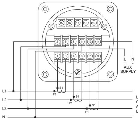
Voltage lines and auxiliary supplied must be fused - see above.
