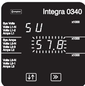
Initially all the digits of the current value will be flashing and the decimal point position illuminated. This is to indicate that initially the "multiplier" must be selected, pressing "↕ Adjust" will move the decimal point position to the right.
