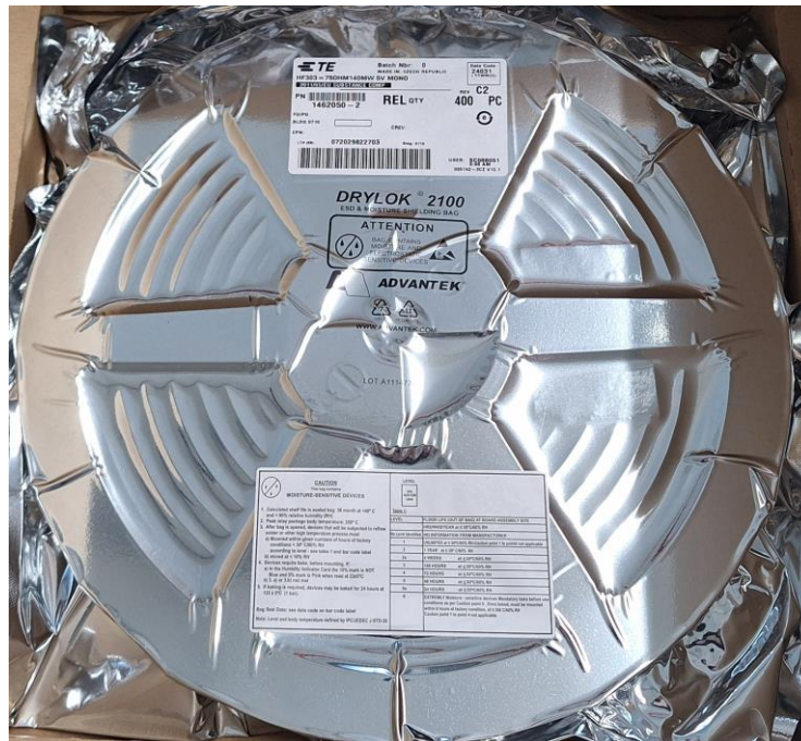
Figure 64: Vacuum bag label position
