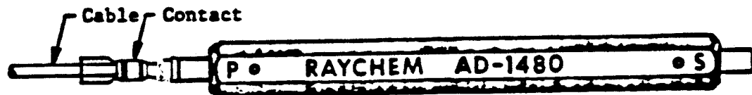
Figure 9 AD-1480 REPAIR HOLDING FIXTURE WITH CONTACT/CABLE ASSEMBLY (OUTER PIN CONTACT SHOWN FOR REFERENCE)
