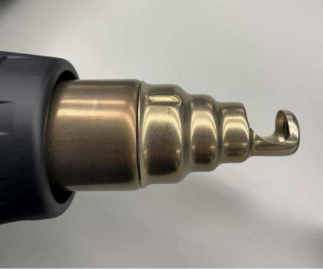
**Figure 16** HL SOLDER SLV REFLECTOR
