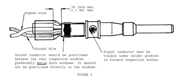
5.2.3 If the wires cannot be positioned correctly, remove them and check for improper strip dimensions, splayed or bent conductors, excess solder on conductors.
