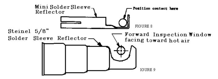
5.3.8 Continue to direct hot air around the forward inspection window while watching the small solder preform.
