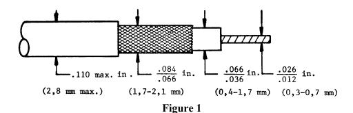
4.2.2 D-602-0172 and D-602-0173 contacts will accommodate coaxial cable of the dimensions shown when the braid is folded back.
