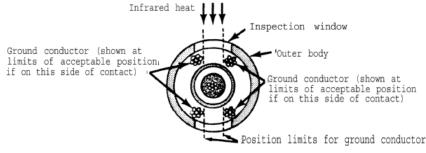
Figure 12A. Positioning of Ground Conductor During Infrared Heating
