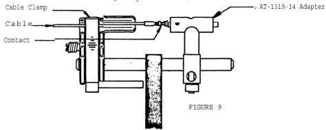
AD-1319 HOLDING FIXTURE AND AT-1319-14 ADAPTER WITH CONTACT/CABLE ASSEMBLY
