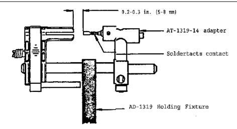
SET-UP DIMENSIONS FOR AD-1319 HOLDING FIXTURE FIGURE 8
