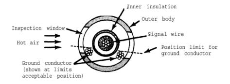
Figure 10A. Positioning of Ground Conductor During Hot Air Heating
