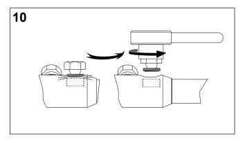
Smooth out any sharp edges of protruding bolts where appropriate by filling it using small piece of yellow tape cut of from of the long tape. Clean and degrease the connector area and the insulation with a cleaning wipe.
