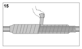
Fix the copper mesh and the screen wires in place with a roll spring close to the end of the joint area. Tighten the roll spring with a twisting action. Cover any sharp edges with adhesive tape.
