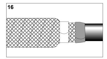
Clean and degrease the ends of the oversheath for a length of about 150 mm.
