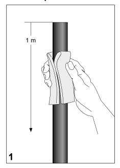
Clean and degrease the end of the oversheath for a length of 1 metre.
