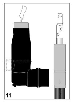
Apply the remaining 50 % of the assembly paste packet onto the inner surface.
