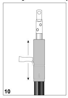
Ensure a clean surface of the stress cone, clean if necessary.
