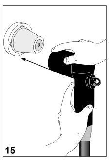
Align the front of the connector body with bushing centre and push the connector onto the bushing.
