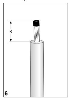
Cut back insulation according to the dimension **K** given in **Table 2**.
