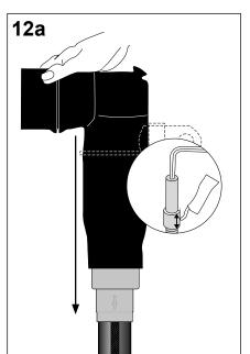
b. Check alignment of the cable lug hole and the elbow body before installing the contact pin.
