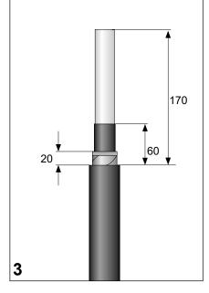
Remove the oversheath over a distance of 170 mm.
