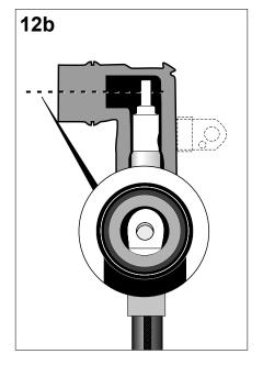
c. Insert the contact pin into the lug and fasten it with the Allen key until the Allen key slightly starts to deform (approx. 7 Nm).
