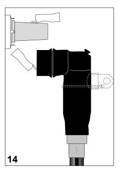
Clean the conical surface of the bushing and the inner surface of the connector.
