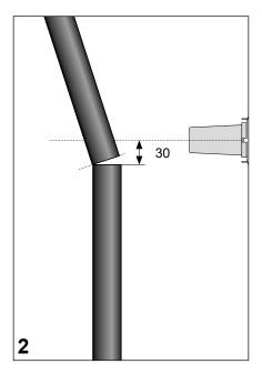
Position the cable with sufficient overlap to the bushing centre line and cut the cable 30 mm below the bushing centre line.
