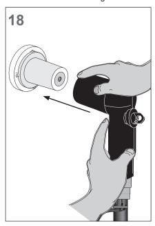
Install the bail restraint centrally behind the connector. Tighten the knurled nuts evenly on both sides and firmly by hand.
