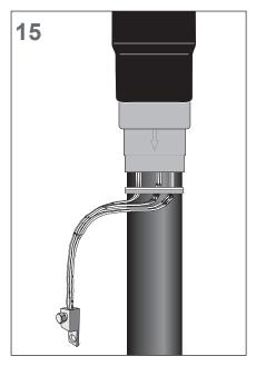
Gather the screen wires together to form an earth lead and cut to same length. Install the screen lug at the end of the screen wires.
