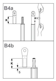
Cut back the insulation according to dimension **K** given in drawing details.
