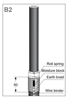
Bind and solder the earth braid to the metal tape shield (or attach the earth lead by any other equivalent method).
