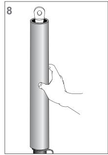
The bottom end of the tubing should be level with the wire binder.
