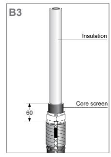
Thoroughly remove the core screen to within 60 mm of the oversheath cut.
