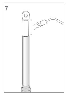
Preheat the cable lug slightly before placing the tubing over the core.
