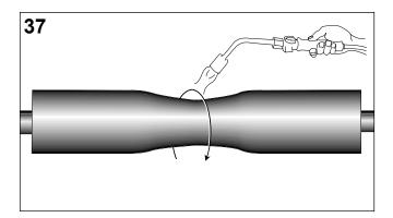
Place the wraparound centrally over the shrunk tubes. Close it at the metal channel.
