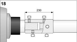
Protect the cable insulation temporarily with non-adhesive tape.
