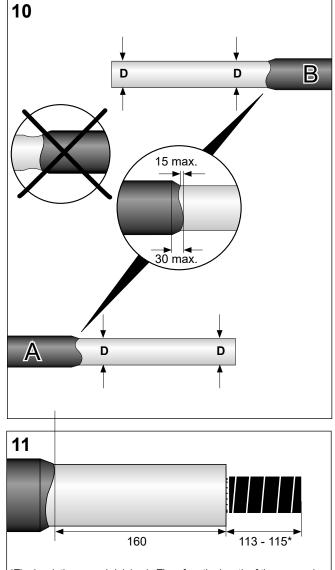
\*The insulation may shrink back. Therefore the length of the exposed conductor may vary from 113 to 115 mm.
