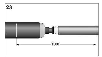
Position the joint centrally over the connector. The distance between the joint body center mark and the Ref. 2 mark on the outer sheath is 1500 mm.
