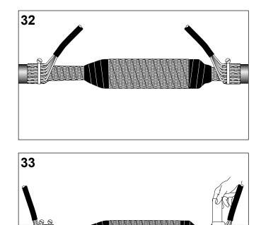
Fold the earth leads back over the worm drive clamp and apply a second worm drive clamp.
