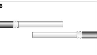
Straight the cable end in the installation position and fix it. Heat the entire cable by applying a heating device to the outer jacket. Before stripping to the required dimensions the cable needs to be cooled down to ambient temperature using slide rails.
