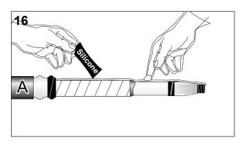
Thoroughly lubricate the cable insulation and PVC tape on cable side  $\mathbf{A}$ .
