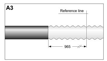
Remove the corrugated copper sheath armour 80 mm from the oversheath cut.
