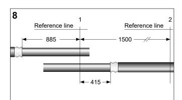
Thoroughly remove the core screen 275 mm from the reference line. The surface of the insulation shall be free from all traces of conductive material.
