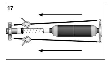
Fit the conductors into the connector so that the connector ends are in close contact to the insulation. (Do not shear off the bolt heads at this stage)
