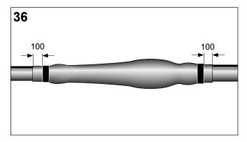
around the cable. Do not cover the exposed shield wires.
