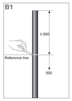
Mark a reference line on the oversheath. The cable has to be ≥ 900 mm above the reference line.
