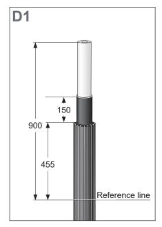
Thoroughly remove the core screen to within 150 mm from the cable outer jacket cut. Make sure the cutting depth of the stripping tool is adjusted accurately so it removes the core screen entirely but does not cut into the insulation.
