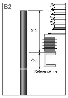
Measure and cut the cable 640 mm above the upper edge of the support rack. The cut must be right angled.
