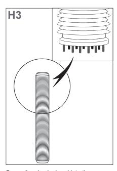
Screw the pins by hand into the insulator to the max. limit. Check that all pins are screed in up to the same lenght.
