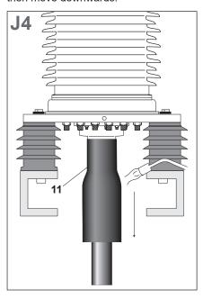
The tubing is fully shrunk when the outer surface is smooth, has a glossy appearance and a flow of sealant is visible at each open end. Intimate surface contact should be made along the whole tubing length, conforming to the profile of the components underneath. The tubing should be smooth and wrinkle free with inner components clearly defined.
