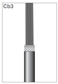
Clean the Al-foil from traces of the outer jacket (if any). Apply the copper mesh on the Al-foil with a CU wire binder. Remove the outer jacket, foil and bedding from the remaining cable end.
