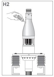
Make sure the O-ring (grey) is applied to the connector stud and into the notch of the base plate. Clean and degrease the gray cover part of the stress cone with alcohol.
