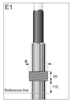
**Starting 115 mm above the reference line,** apply a 50 mm wide packing of cotton cloth tape.
