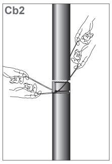
Cut through the outer jacket with the supplied string. Remove the outer jacket from the Al-foil by slicing segments away with the string as shown in the picture.
