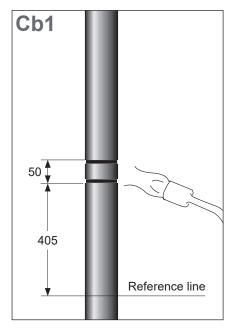
Heat the cable outer jacket 405 mm above the reference line. Soften approx. 50 mm of the surface.
