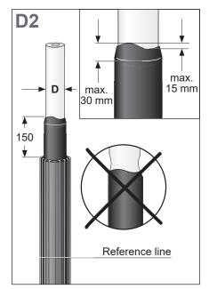
Chamfer the outer semicon layer on the cut between 20 - 30 mm.
