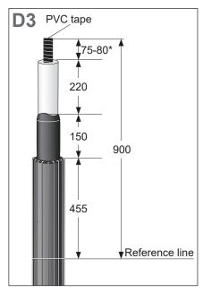
Remove the insulation as shown in the drawing. Slightly smooth the insulation edge.
