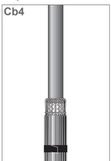
Place a roll spring over the shield wires. Fix the roll spring by twisting.
