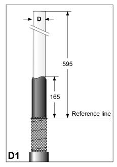
Thoroughly remove the outer semicon layer to within 165 mm above the reference line until the diameter of the insulation is **D** (see **Table 1**).
