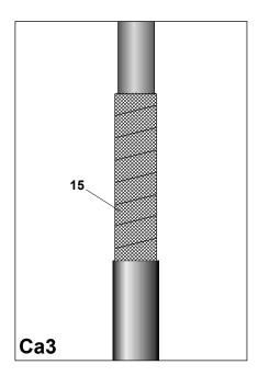
Apply 3 layers of copper mesh (15) onto the Al wires.
