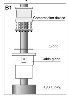
Move the heat shrinkable thick wall tubing, cable gland, O-ring and compression device down the cable jacket as shown in the drawing.
