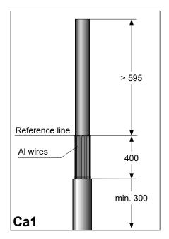
Remove the oversheath up to 400 mm below the reference line.
