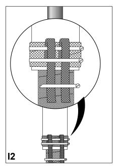
Remove the PVC tape and bend down the copper braids. Fasten the copper braids with a second armour clamp on the cable gland.
