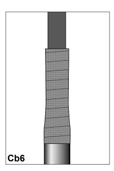
Apply 3 layers of Cu-mesh onto the Al wires and the metal foil.
