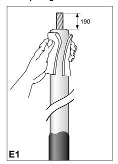
Remove 190 mm of the cable insulation as shown.
