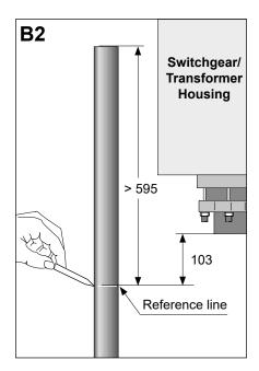
Mark the reference line on the cable 103 mm below the transformer housing as shown.
