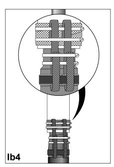
Fasten the copper braids with the last armour clamp as shown.
