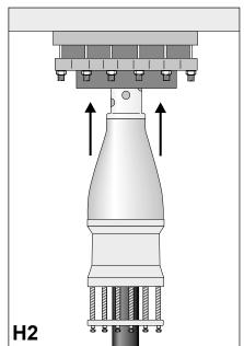
Push the cable with the male plug-in unit in a straight line into the epoxy insulator.
