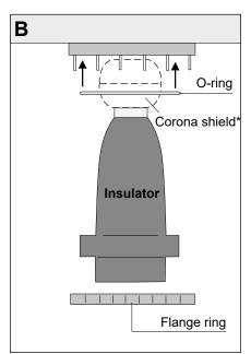
Put the O-ring (supplied by the switchgear/transformer manufacturer) into the sealing groove of the switch gear. Clean and degrease the epoxy insulator (5). Keep it free from dust and dirt.
