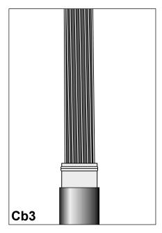
Fix the metal foil with a wire binder. Clean the metal foil from traces of the outer jacket (if any). Remove the outer jacket, foil and bedding from the remaining cable end.
