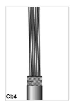
Wrap 3 layers of Cu-mesh over the metal foil.
