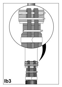
Fix the copper braids onto the metal foil using a roll spring.
