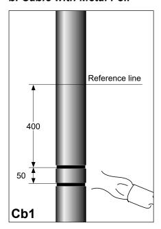
Heat the cable outer jacket 400 mm below the reference line. Soften approx. 50 mm of the surface.
