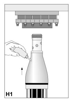
Remove the temporary protection from the connector stud. Clean and degrease the silicone stress cone with alcohol.
