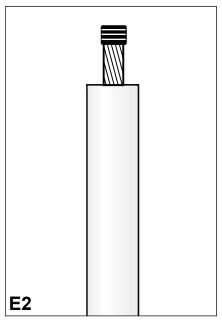
Protect the conductor with PVC tape as shown.
