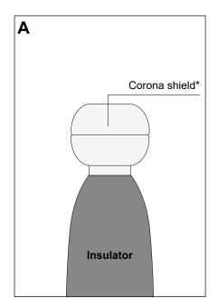
Bolt the lower part of the corona shield to the insulator electrode. Apply the top part of the corona shield.
