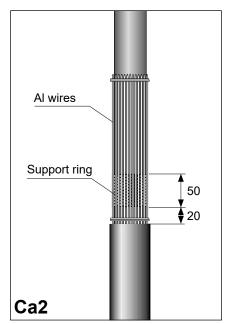
Slide the support ring under the Al wires. Position the support ring 20 mm above the outer sheath cut.
