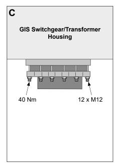
Insert the epoxy insulator into the switchgear/transformer housing. Apply the fixing ring. Bolt the fixing ring evenly to the switchgear/transformer housing.
