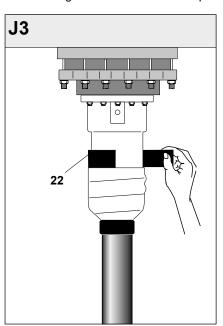
Position the heat shrinkable thick wall tubing approx. 150 mm on the cable gland.
