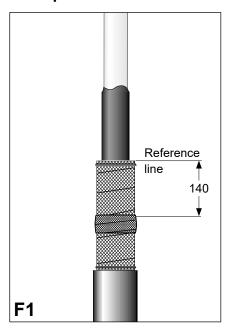
Apply a 50 mm wide packing of textile tape. Start wrapping **140 mm below the reference line** as shown in the drawing.
