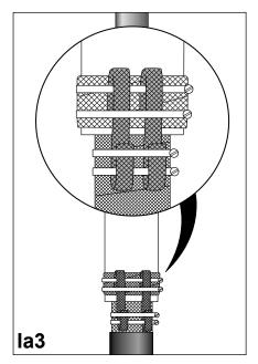
Fasten the copper braids with the last armour clamp as shown.
