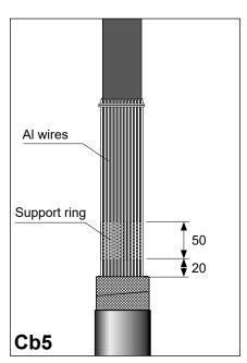
Slide the support ring under the Al wires. Position the support ring 20 mm above the outer sheath cut.
