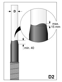
**Chamfer the outer semicon layer** at least 40 mm.
