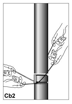
Cut through the outer jacket with the supplied string. Remove the outer jacket from the metal foil by slicing segments away with the string as shown in the drawing.
