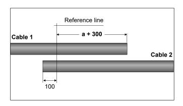
Cable Preparation Dimensions in mm
