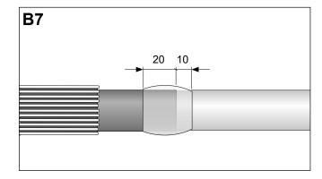
Remove the printed release paper from the void filling tape (yellow). Apply the tape with a 50 % overlap stretching it to about half of its original width.
