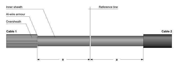
Remove the oversheath of both cables to dimension  $\bf a$ , measured from the reference line. Clean the remaining oversheath of both cables for about 600 mm.
