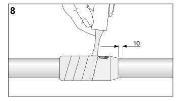
Pull the stress control sleeve (black) from the inside of the tubing set and position it centrally over the connector. Start shrinking in the centre working towards the ends. The tubing should be fully shrunk and wrinkle free.
