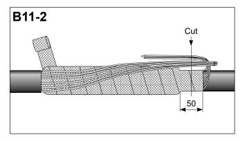
Connect the shield wires by crimping or any other equivalent method.
