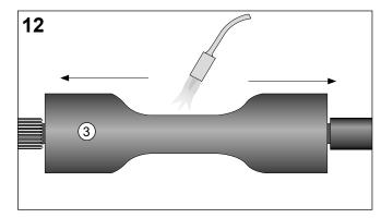
Carefully remove 100 mm of the oversheath on cable 2. Do not cut the armour wires.
