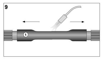
Position the screened insulating sleeve (black and red) centrally over the connector area.
