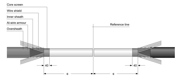
Remove the inner sheath to dimension  $\mathbf{c}$  (see **table 3**). Bend back the shield wires onto the oversheath. Cover the sharp wire ends with plastic tape. Cut the cores at the reference line.
