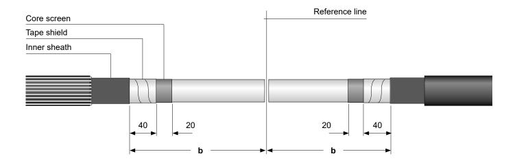
Cut the cores at the reference line. Remove the inner sheath to dimension **b** (see **table 3**).
