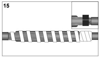
Position the outer sealing sleeve centrally, then shrink the outer sleeve (black) down starting in the centre and working towards the ends.
