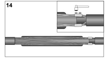
Wrap a piece of the inner bedding or of the cable sheath over the connectors.
