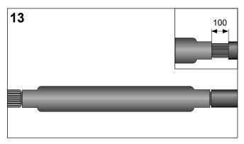
Thoroughly clean the armour wires from cable 1. Separate the armour wires and form equal bunches, according to the number of the mechanical connectors supplied with the kit.
