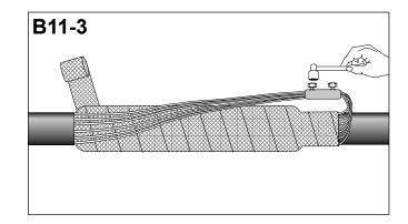
Centre the inner sealing sleeve (black) over the joint area. Start shrinking in the centre, working towards the ends. This sleeve is to seal on to the cable inner sheath.
