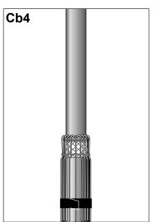
Install the roll spring around the shield wires. Tighten the roll spring with a twisting action. Remove the wire binder which is near the cable oversheath.
