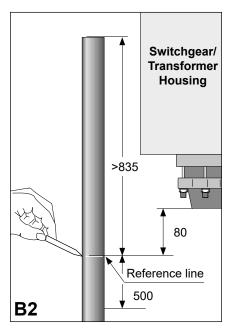
Mark the reference line on the cable 80 mm below the transformer switchgear housing as shown.
