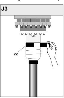
Position the heat shrinkable thick wall tubing directly below the grounding point. Shrink the tube into place. Start shrinking at the top then move downwards.
