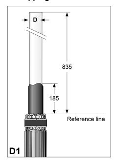
Thoroughly remove the outer semicon layer to within 185 mm above the reference line until the diameter of the insulation is **D** (see **Table 1**).
