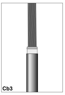
Fix the Al-foil with a wire binder. Clean the Al-foil from traces of the outer jacket (if any). Remove the outer jacket, foil and bedding from the remaining cable end.
