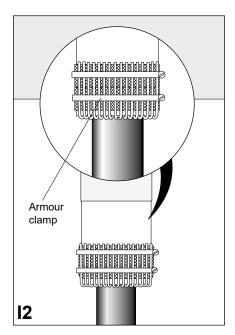
Cut the shield wires and bend them back onto the cable gland. Fix the shield wires as shown using two armour clamps.
