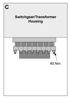
Insert the epoxy insulator into the switchgear/transformer housing. Apply the fixing ring. Bolt the fixing ring evenly to the switchgear/transformer housing. Make sure the cantilever force applied to the epoxy bushing is low!
