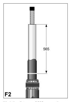
Mark the distance of 565 mm on the semicon tape measured from the insulation cut as shown in the drawing.
