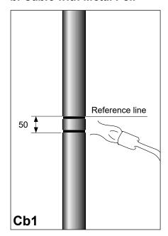
Heat the cable outer jacket below the reference line. Soften approx. 50 mm of the surface.
