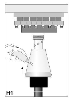
Remove the temporary protection from the connector stud. Clean and degrease the transparent cover part of the silicone stress cone with alcohol.
