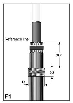
**360 mm below the reference line,** apply a 50 mm wide packing of cotton cloth tape.
