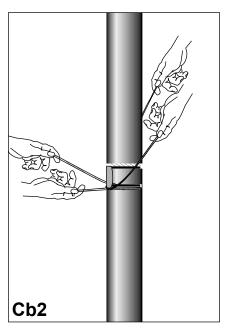
Cut through the outer jacket with the supplied string. Remove the outer jacket from the Al-foil (by slicing segments away with the string as shown in the picture.
