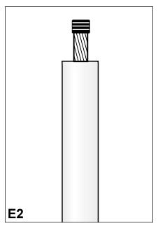
Protect the conductor with PVC tape as shown.
