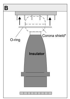
Put the O-ring (supplied by the switchgear/transformer manufacturer) into the sealing groove of the switch gear. Clean and degrease the epoxy insulator. Keep it free from dust and dirt.
