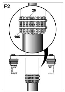
Bend the copper wires (105) back.
