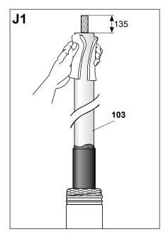
Remove the cable insulation (103) for a length of 135 mm.
