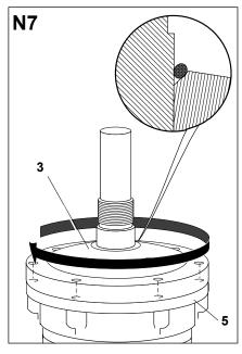
Screw the top plate (3) and sealing ring down until the top plate touches the flange of the composite insulator (5). Turn the top plate one more turn. Make sure its holes are in line with the holes of the composite insulator. Grease the O-ring.
