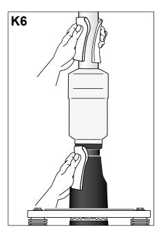
Clean the cable and all parts installed.
