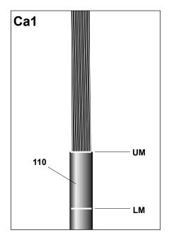
Starting from the upper mark (**UM**), remove the outer jacket (**110**) of the cable as shown.
