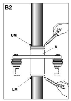
On the cable, mark the upper mark (UM) next to the uppermost edge and the lower mark (LM) next to the lowermost edge of the cable gland (8) using a marking pen or PVC tape as shown. Make sure that the remaining cable length above UM is greater than L.
