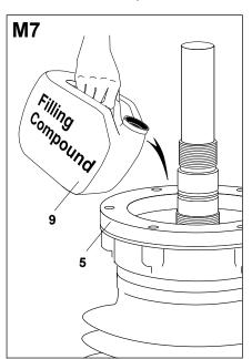
Check the filling level. Make sure the filling compound level is 300 mm below the top of the composite insulator (5).
