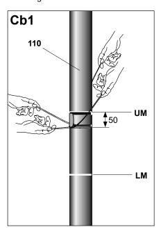
Fix the Al foil (106) with a wire binder (25). Clean the Al foil from traces of the outer jacket (if there are any).
