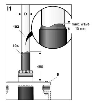
Remove the outer semicon layer (104) to within 480 mm from the base plate (6).
