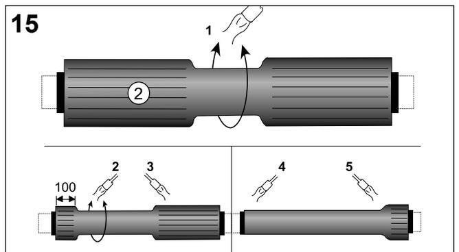
Starting from the branch side, apply the copper mesh with a 50% overlap around the previously installed tube so that the whole joint area is covered.
