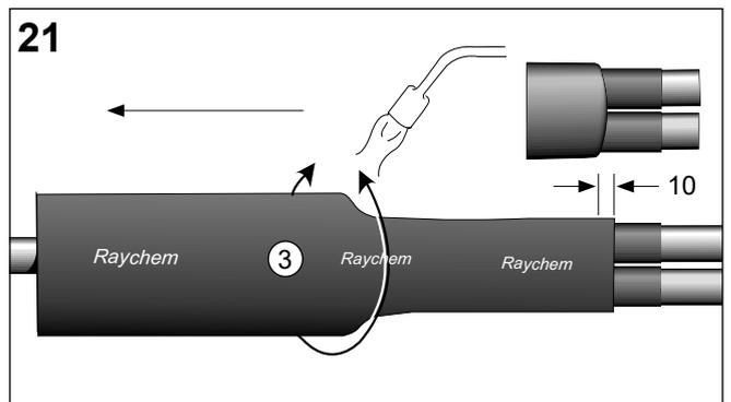
Secure the main and branch cable close to the joint area with a cable tie or PVC tape and allow the joint to cool before applying any mechanical strain.
