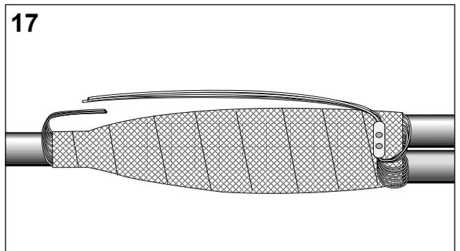
Form an earth lead of the shield wires and insert both ends into the second mechanical shield connector supplied.
