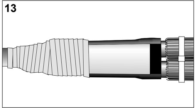
Pull the stress control tubing (black) from inside the tubing set and position it with 10 mm overlap at the rubber profile. Start shrinking from the branch cable side working towards the single core side. The tubing should be fully shrunk and wrinkle free.
