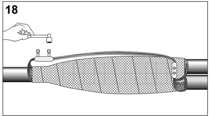
Wrap a second layer of copper mesh round the joint with a 50% overlap. Cover the complete joint area including the mechanical shield connector.
