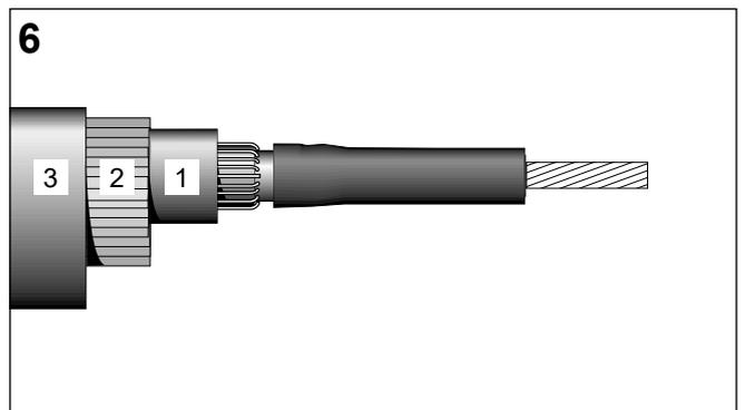
Slide the breakout (breakout fingers first) over the cables on the branch side of the joint.
