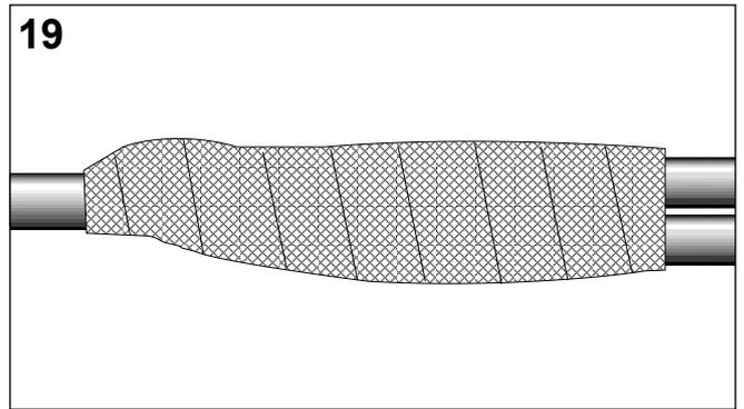
Clean and degrease all oversheath ends. Push the breakout down into the crutch. Shrink it into place starting at the centre. The numbers in the drawing indicate the shrink sequence.
