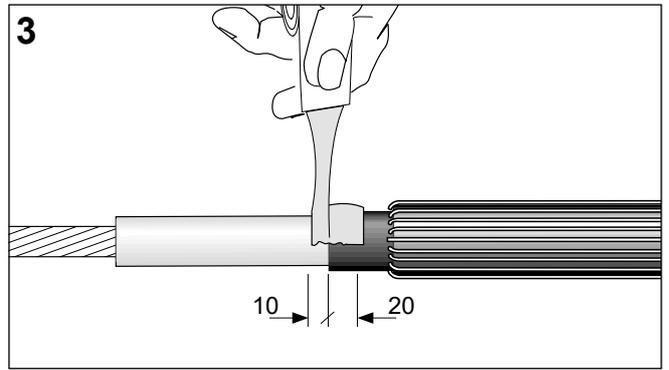
Position the stress control tubing (black) level with the insulation cutback. Shrink the tubing into position starting at the insulation cutback working towards the oversheath as shown in the drawing.
