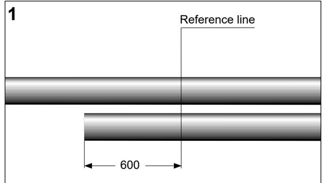
Position the short build up sleeve **on the single core side** level with the end of the oversheath as shown in drawing 2.
