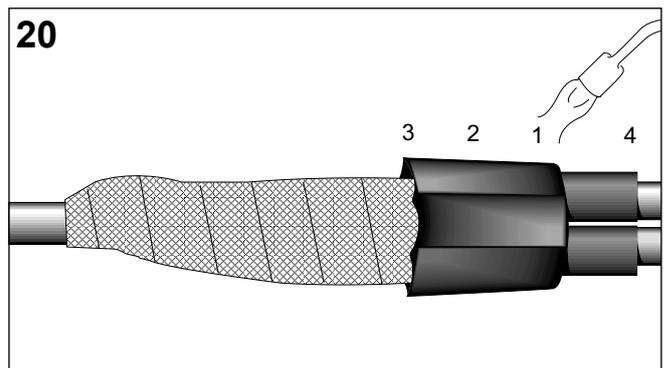
Position the outer sealing sleeve across the joint overlapping the base of the breakout turrets for 10 mm as shown in the drawing. Start shrinking from the branch cable side working towards the single core cable side.
