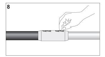
Remove the release paper from the void filling tape (yellow). Apply the tape with a 50 % overlap stretching it to about half of its original width.
