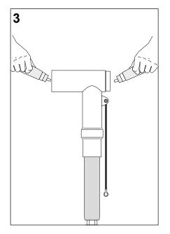
Align the eye of the surge arrestor lug with the threaded pin and push the screened surge arrester onto the bushing.
