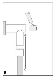
Clean the inner surface of the back end and apply a thin layer of assembly grease. Do the same with the conical interface of the back plug as shown.
