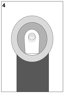
Insert the spring washer and hex nut. Tighten the hex nut (24 mm) onto the stud with a torque wrench at **30 Nm**.
