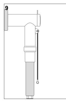
Select the shortest distance to ground and adjust the ground lead of the arrester to that length. Install the lug supplied on the free end of the ground lead.
