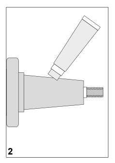
Clean the conical surface of the bushing and lubricate it with the assembly grease as shown.
