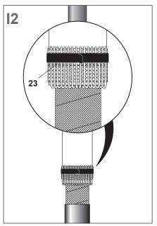
Remove the PVC tape. Fix the three copper braids (24) to the copper wires (105) as shown using two armour clamps (20).
