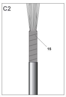
Apply three layers of copper mesh tape (15) onto the lead sheath (107).
