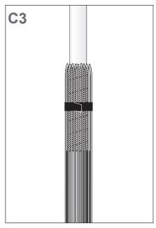
Bend the shield wires back onto the lead sheath and fix them temporarily in place with PVC tape.
