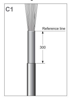
Remove the outer jacket (110) and bedding 300 mm below the reference line.
