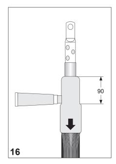
Clean the outer surface of stress cone and apply a thin layer of lubricant onto the outer surface of the stress cone over a length of 90 mm with the sponge top as shown in the drawing.
