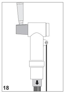
Clean the conical front end of the coupling connector and apply a thin layer of lubricant onto the outer surface of the cone with the sponge top.
