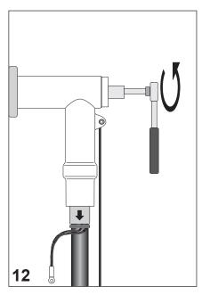
Remove from the installed connector the back plug and save it in a clean container.
