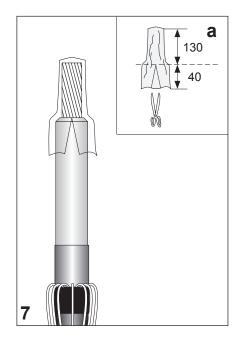
Cut the small protective bag (assembly aid) at the bottom end at a length of 40 mm on one side (see detail **a**).
