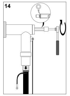
Insert the **threaded stud M16** into the rear end of the coupling stud and tighten it up with an Allen key (8 mm). Maximum torque: **30 Nm**.
