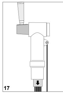
Clean the conical front end of the coupling connector and apply a thin layer of lubricant onto the outer surface of the cone with the sponge top. Continue immediately with the next step.
