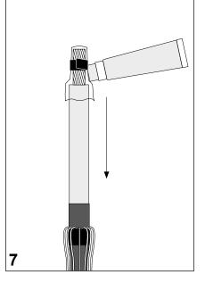
Slide the small protective bag (assembly aid) over the exposed conductor and tie it down with a PVC tape as shown in the drawing.
