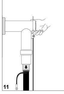
Remove from the installed connector the conductive endcap and save it in a clean container.
