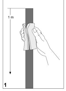
Clean and degrease the end of the oversheath for a length of 1 metre with solvent wipe.
