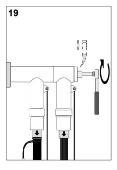
Clean the inner surface of connector back end and apply a thin layer of assembly lubricant. Do the same with the conical interface of the back plug as shown in detail.
