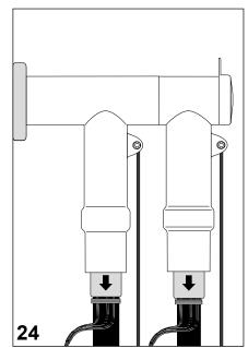
Screened separable coupling connector completed.
