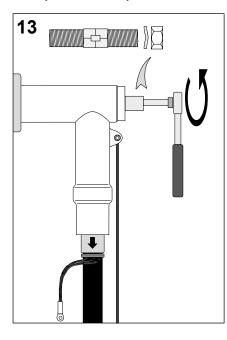
Insert coupling stud with tinned Cuwasher (see detail) into the rear end of the connector and tighten it up with a torque wrench (27 mm).
