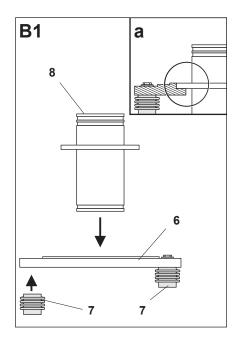
Temporarily fix the support insulators (7) to the base plate (6) with the larger screws.
