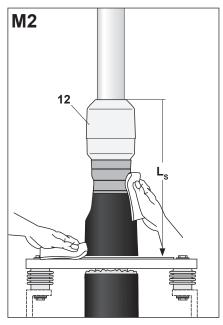
Remove the protection materials from the stress cone (12).
