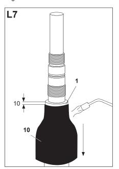
The tube is fully shrunk when the outer surface is smooth, has a glossy appearance and a flow of sealant is visible at each open end.
