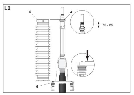
Check the distance between the base plate (6) and the top of the support nut (4). Adjust the distance exactly to the height of the composite insulator (5). If this is not possible, rework the cable.
