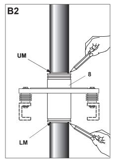
Mark on the cable the upper mark (UM) next to the uppermost edge and the lower mark (LM) next to the lowermost edge of the cable gland (8) using a marking pen or PVC tape as shown. Make sure that the remaining cable length above UM is greater than L.
