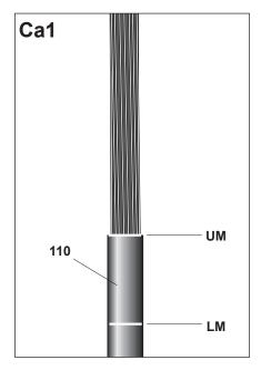
Starting out from the upper mark (**UM**), remove the outer jacket (**110**) of the cable as shown.
