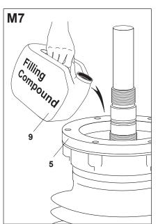
Check the filling level. Make sure the filling compound level is 100 mm below the top of the composite insulator (5).
