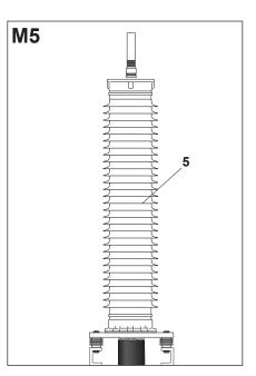
Carefully slide the composite insulator (5) over the cable assembly, the larger bottom flange first.
