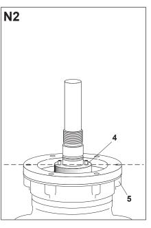
Adjust the support nut (4) temporarily so its surface **is flush with** the top of the composite insulator (5).
