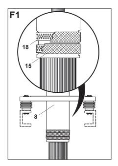
Abrade, degrease and clean the cable gland (8).
