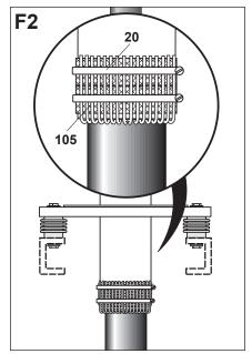
Bend the copper wires (105) back.
