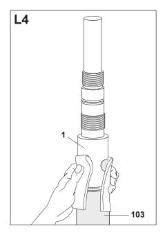
Degrease and clean the lug (1) and the cable insulation (103).
