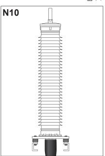
Fix the top plate (3) to the composite insulator (5) as shown in the detail. Use a torque of 55 Nm.
