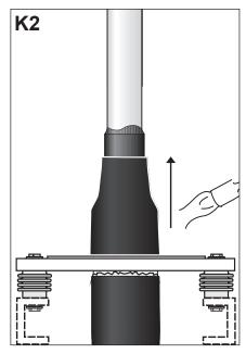
Slide the short **uncoated** heat-shrink tube (**length 200 mm**) over the cable down to the base plate and shrink it into place.
