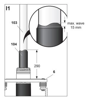
Remove the outer semicon layer (104) to within 290 mm from the base plate (6).
