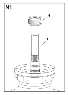
Grease the support nut (4) with silicone grease. Slide the support nut over the lug (1).
