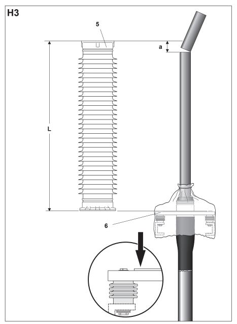
Measure the height L of the composite insulator (5).
