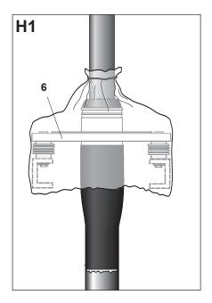
Protect the base plate (6) with plastic foil.
