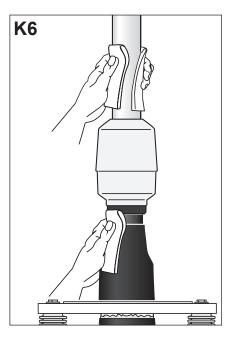
Clean the cable and all parts installed.
