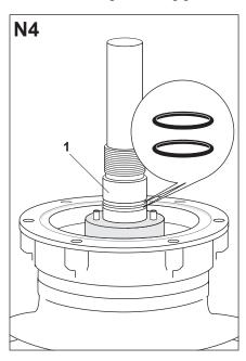
Place the sealing ring in the groove of the housing flange. Grease the O-rings with silicone grease.
