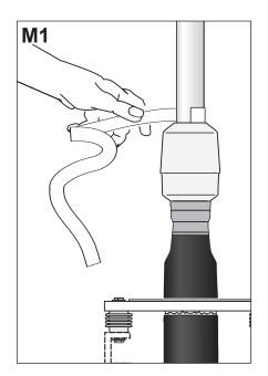
Remove the transparent tape from above the stress cone.
