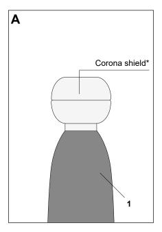
Bolt the corona shield to the insulator electrode.
