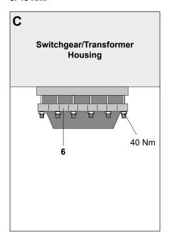
Install the insulator to the switchgear/ transformer housing.
