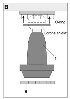
Put the O-ring (supplied by the switchgear/transformer manufacturer) into the sealing groove of the switchgear. Clean and degrease the epoxy insulator (1). Keep it free from dust and dirt.
