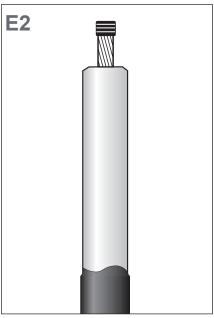
Protect the conductor (101) with PVC tape (23) as shown.
