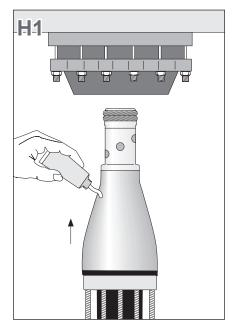
Remove the temporary protection from the connector stud. Clean and degrease the transparent cover part of the silicone stress cone (12) with alcohol.
