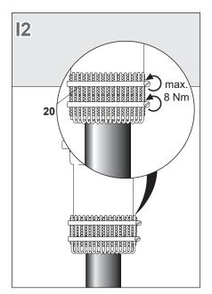
Cut the shield wires and bend them back onto the cable gland. Fix the shield wires as shown using two armour clamps (20) with the defined torque of maximally 8 Nm.
