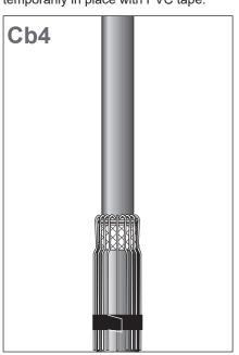
Install the roll spring (19) around the shield wires. Tighten the roll spring with a twisting action.
