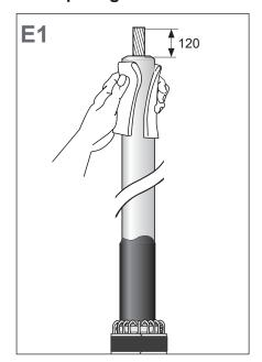
Remove 120 mm of the cable insulation (103) as shown.
