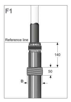
140 mm below the reference line, apply a 50 mm wide packing of textile tape (21).
