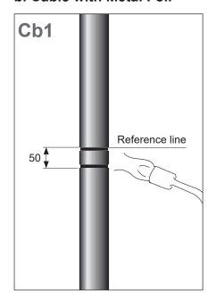
Heat the cable oversheath (130) below the reference line. Soften approx. 50 mm of the surface.
