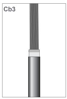
Fix the Al-foil (106) with a wire binder. Clean the Al-foil from traces of the outer jacket (if any). Remove the oversheath, foil and bedding from the remaining cable end.
