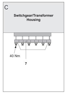
Insert the epoxy insulator (5) into the switchgear/transformer housing. Apply the fixing ring (7). Bolt the flange evenly to the switchgear/transformer housing.
