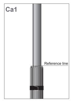
Starting out from the reference line, remove the outer jacket of the cable as shown.
