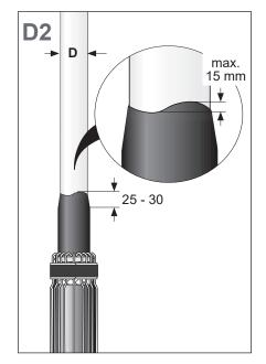
**Chamfer the outer semicon layer** in between 25 to 30 mm.
