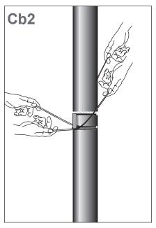
Cut through the oversheath (130) with the supplied string. Remove the outer jacket from the Al-foil (106) by slicing segments away with the string as shown in the picture.
