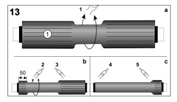
Starting with a 50 mm overlap onto the oversheath of the cable side with the short shield wires, wrap one layer of copper mesh round the joint with a 50% overlap.
