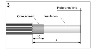
Remove the insulation on both cores equal to the insert depth I (see Table 1).
