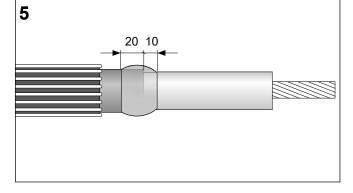
Slide the stress control tubing (black) over the plastic cable core level with the end of the insulation cut back.
