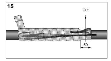
Form an earth lead of the shield wires and insert both ends into the mechanical shield connector supplied.
