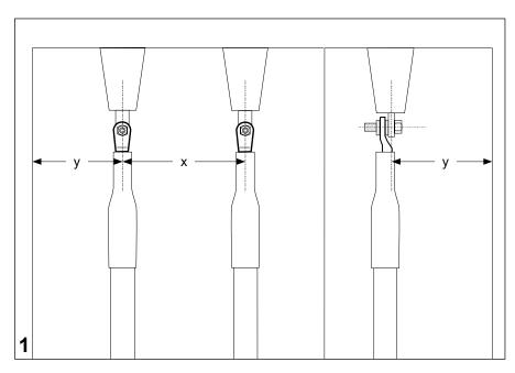
Ensure that the minimum clearances with the insulating RCAB boot are as follows:
