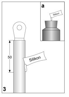
Clean the upper side of the termination and inside of the shrouded termination boot (large diameter).
