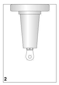
Install the universal terminal screw with counter nut into the bushing.
