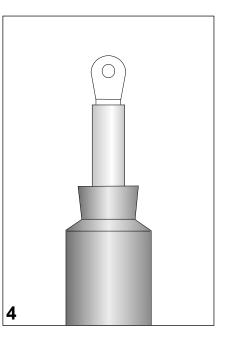
Starting with the small diameter of the boot slide the RCAB over the termination.
