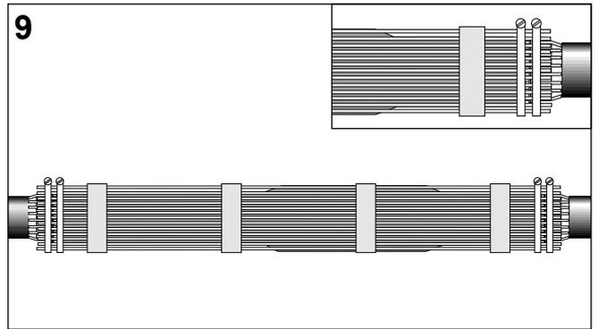
Clean and degrease the ends of the oversheath for a length of about 150 mm. Position the top sealing sleeve over the short core end so that it overlaps the end of the oversheath by about 150 mm. Start shrinking at the oversheath end, working towards the connector area.
