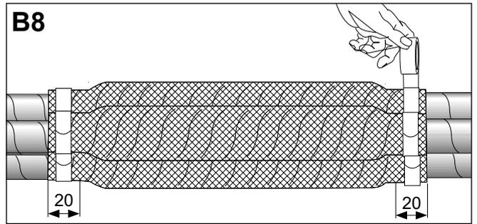
Wrap the joint case round the joint and secure with cloth tape as shown in the picture. Clamp the ends of the joint case onto the steel wire armour using the screw clips. Cover the sharp edges of the screw clips by fastening a piece of cable oversheath over the screw with the remaining cloth tape.
