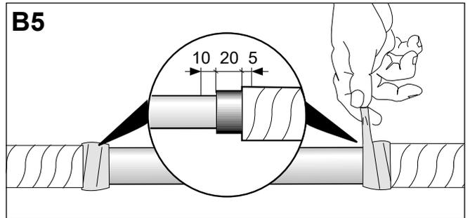
Position **all three** stress control sleeves (black) centrally over the connectors. Start shrinking in the centre working towards the ends. The sleeves should be fully shrunk and wrinkle free.
