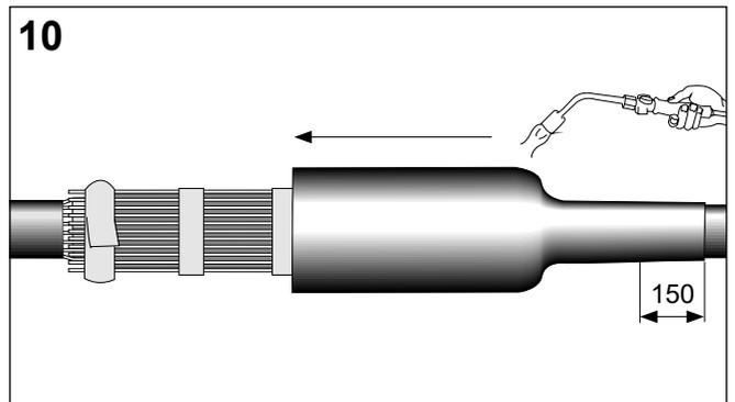
Position the second sealing sleeve so that it overlaps the other end of the oversheath by 150 mm. Start shrinking at the oversheath end, working towards the connector area.
