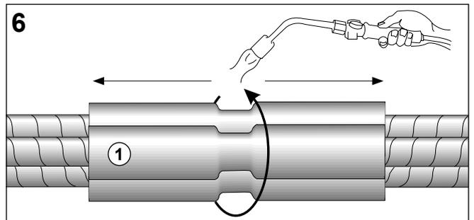
Position **all three** screened insulating sleeves (black and red) centrally over the previously installed tubing.
