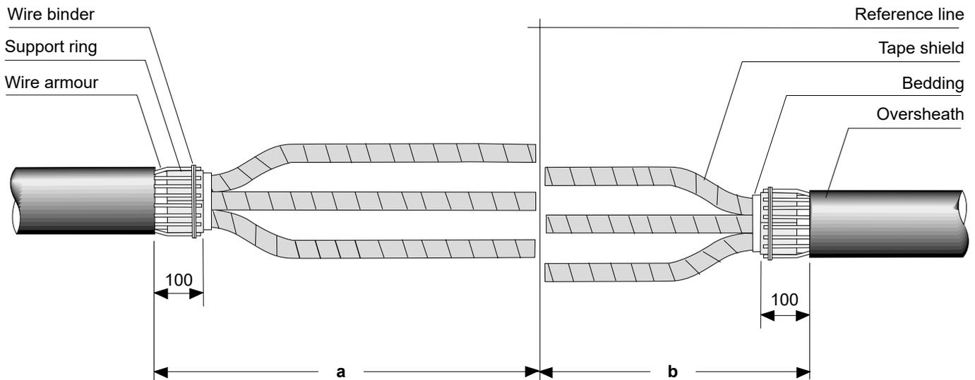
Remove the oversheath, armour and bedding according to the dimensions given in drawing **A**.
