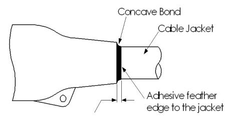
This dimension approximately equivalent to the boot or tubing wall thickness
