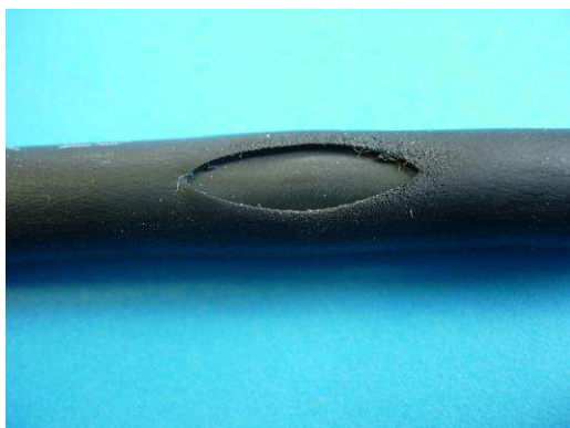
NOT ACCEPTABLE Tubing Split
