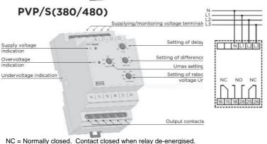
NO = Normally open. Contact open when relay de-energised.
